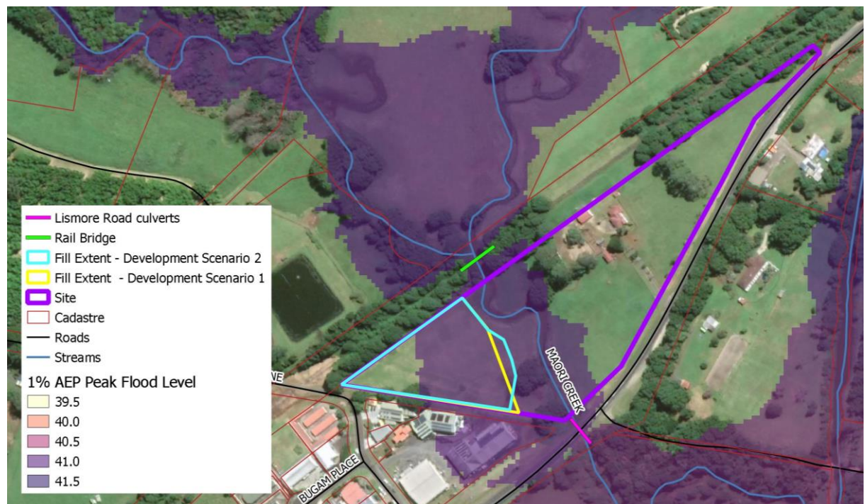
Figure 4-1 Fill Pad Alignments for Development Scenarios
